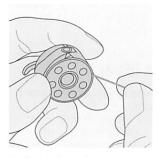
Pull the thread counter clockwise into the slot.
